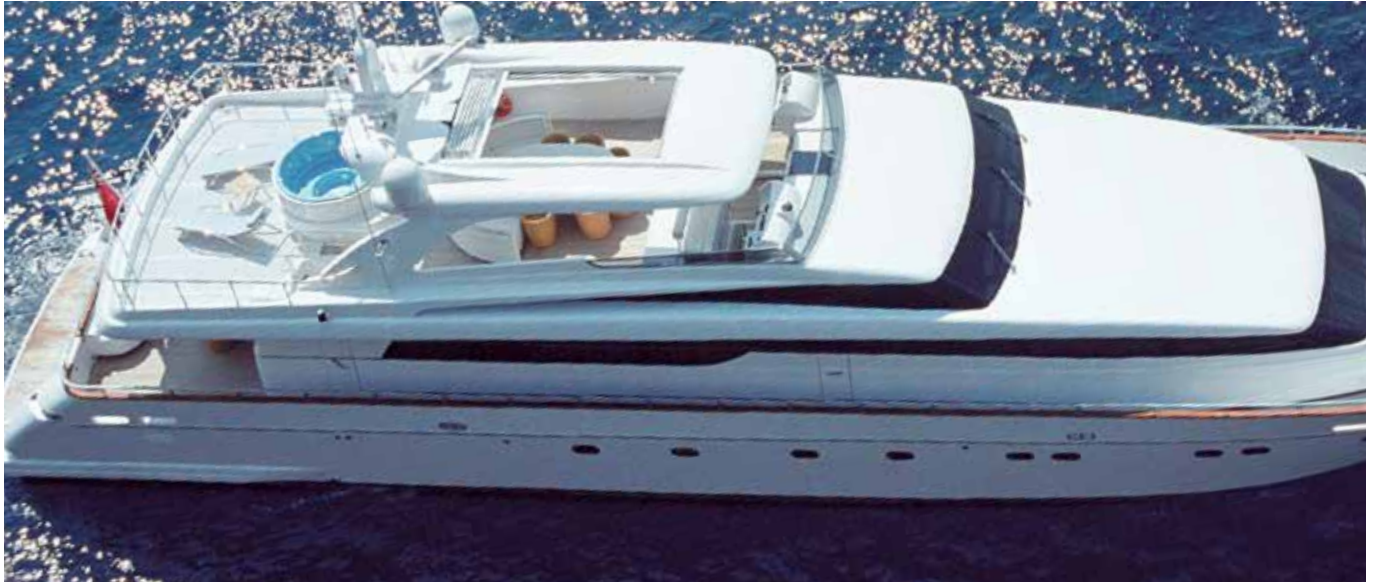
The SL108 yacht (top), from the Sanlorenzo shipbuilding yards, uses Viraver glass panels made with high-resistance SentryGlas® ionoplast interlayer for all frontal and lateral glazing. The structural interlayer was selected due to its ability to withstand both impacts and harsh climates. The laminated glass made with high-resistant SentryGlas® interlayer is also used for Sanlorenzo's SL72, SL82 and SL88 models. © Sanlorenzo.
